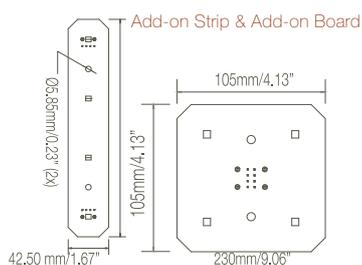
**Medium pixel pitch, wide beam angle** 1PXL Board offers a 62.5 mm pixel pitch and a wide beam angle of 120°, making them efficient tools for low resolution graphics, decorative illumination, or stunning backlighting on varying levels of complexity.
