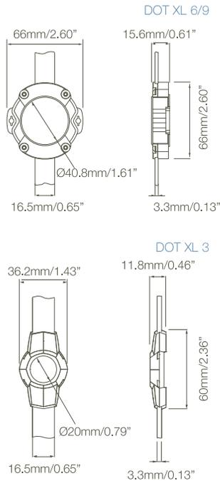
**Various customization options** Dot XL customization choices include number of LEDs per round Dot casing (3, 6, or 9); LED color (RGB, warm white, or cold white); pixel pitch; and diffuser dome.
