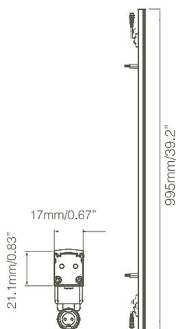
**Sleek, slim profile** The slender fixture housing allows Monochrome Tube to fit into the smallest of installation spaces. Though small and easily hidden from view, Monochrome Tube continues to deliver even strips of white light.
