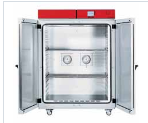
Test cabinet where the temperature can be varied from -20°C to 100°C. By placing numerous sensors, data can be analysed by advanced calculation software.
